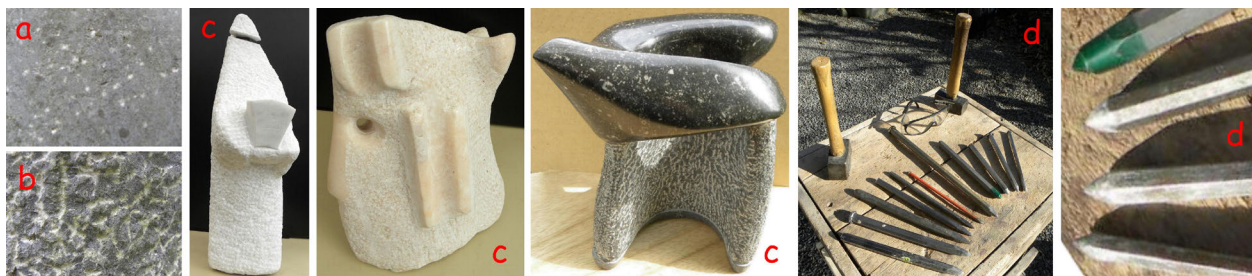
Figure 1. a. Stone bruises or white marks by point chisel; b. point chiseled texture; c. mainly point chiseled works in various kinds of stone; d. point chisels, mallets and safety glasses.
