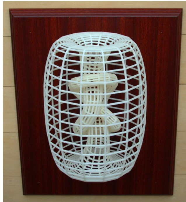
Internally Knotted Figure-8 Torus 8" x 6" x 6" 3D Model made on an FDM machine, ABS plastic
