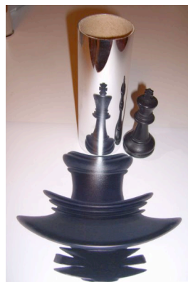
Figure 4: A real chess piece (back right), its anamorphic projection (front) and its virtual image (center).
