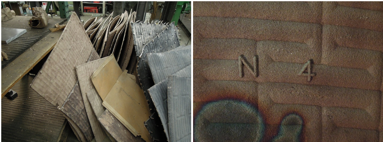
We carved each of the 144 parts in reverse with a set of adjacency labels so that they could be welded together without further instructions or pictures. We sand cast all 144 parts and have welded the top half of 72 parts and the bottom half of 72 parts. The final four photos give an idea of where things are in the Torus Assembly Building.
