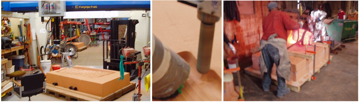
The robot is on the left, middle is the orientable diamond coated cutting tool, right is pouring the bronze into the sandstone molds. This gantry robot has a name, Σταματία = 'fallen angel', it fits.
