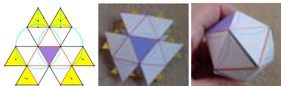
Figure 3: An icosahedron with pivots constructed, assembled, and activated.
